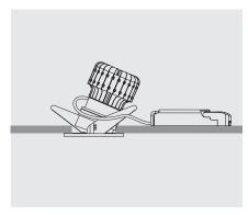
4. Adjust the angle required. Assembly complete.
