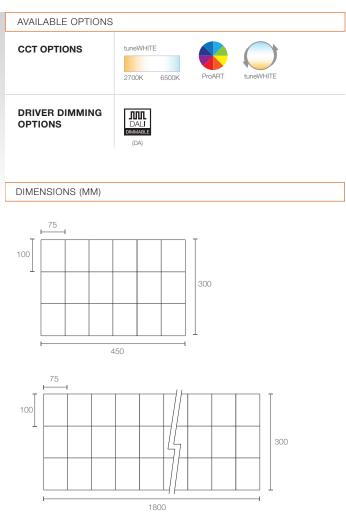
Width x Length x Height : 300mm x 450mm x 1mm
