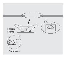
1. Cutout and compress spring plates to insert fixture frame to ceiling.
