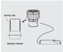
2. Attach module to module holder 3. Gently insert module holder with spring clip and connect module to driver.
