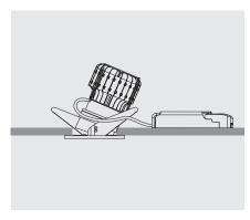
4. Adjust the angle required. Installation complete.
