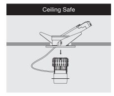
Reverse the installation step 3 for LED module replacement / maintenance.
